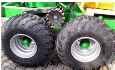
Fig. 104. Non-driven and pinion-driven bogie axle
