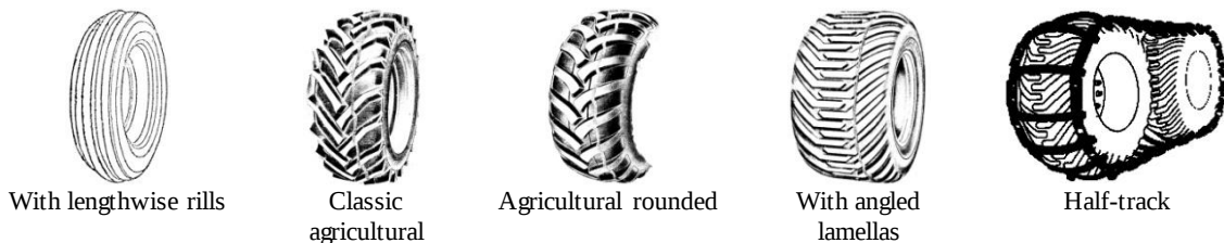
Fig. 12. Patterns of tyre treads and half-track in tyres with angled lamellas
