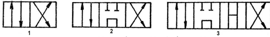
1 – two-position, 2 – three-position, 3 – four-position Fig. 41. Examples of four-way distributor schematics
