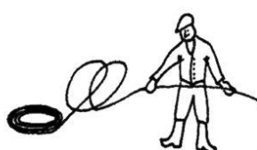
incorrect cable unwinding
