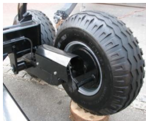
Fig. 104. Non-driven and pinion-driven bogie axle
