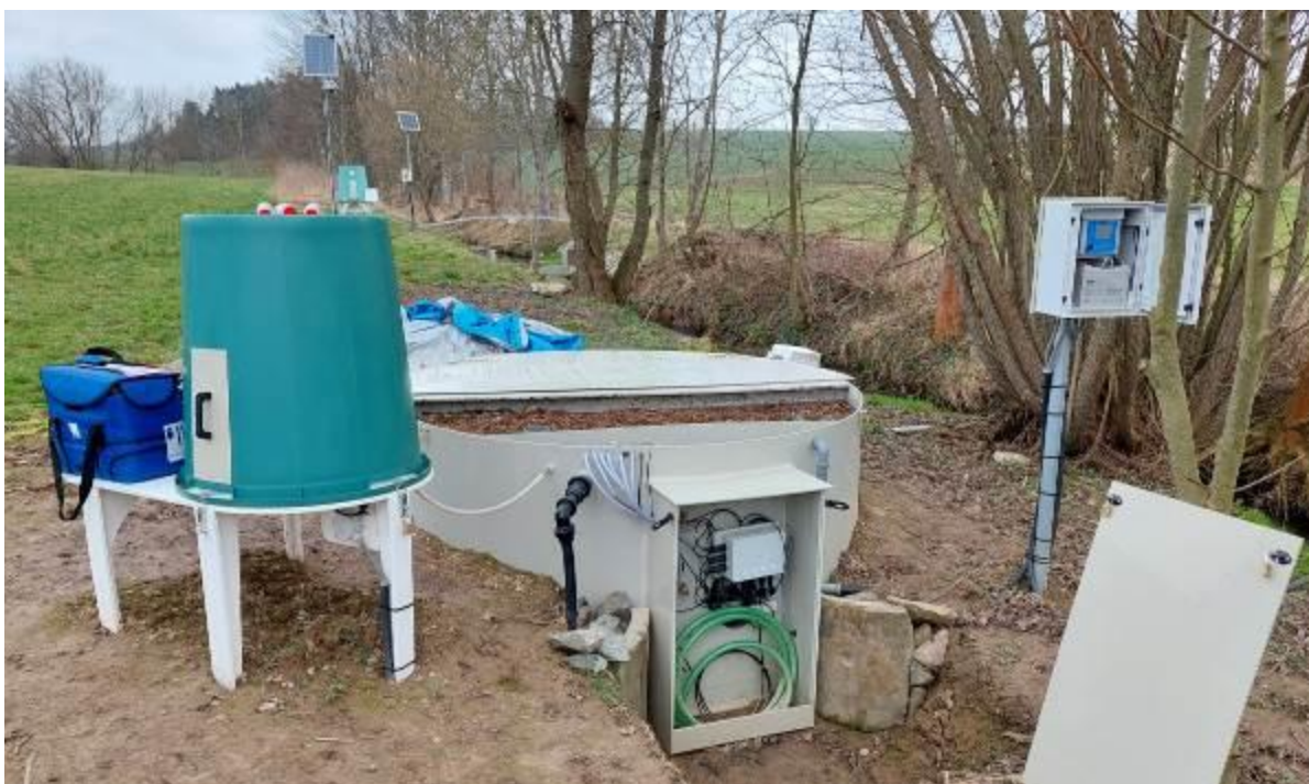
Fig. 2 Combined bioreactor and surrounding equipment (ISCO sampler, telemetry station)
