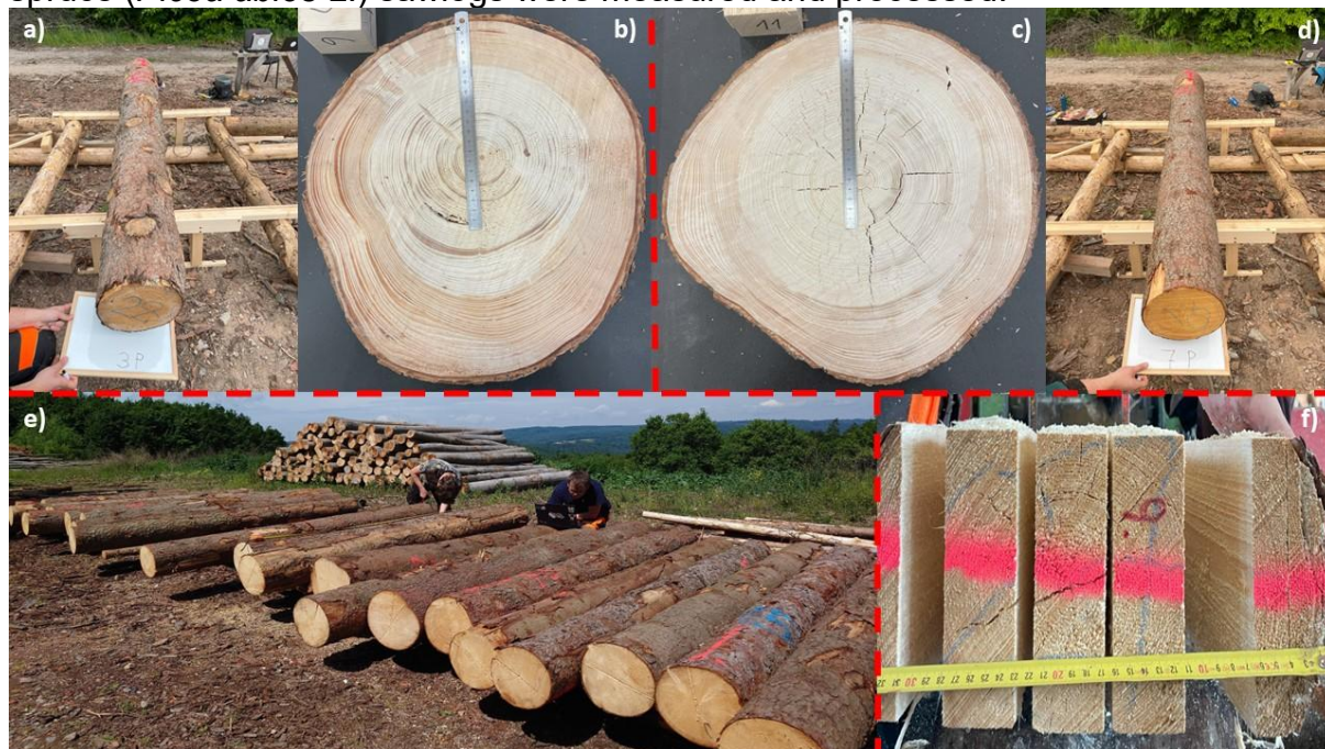
Fig. 5: Low-quality sawlog III.D (a); Sample with a higher MC = 90.4% (b); Sample with a lower MC = 81.9% (c); High-quality sawlog III.A (d); Measuring area at the Sawmill Olomučany (e); Cant sawing with a resulting 3 central boards (f)
